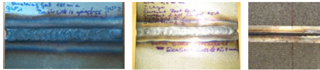
Fig. 1: Welding regions produced by TIG welding (left), plasma welding (middle) and laser welding (right).
