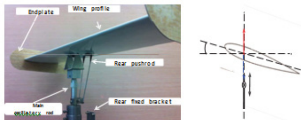
(a) Airfoil model setup and driving mechanism (b) Wing plunging motion schematic diagram
