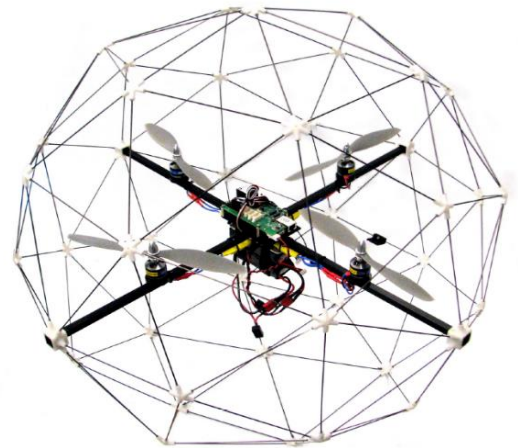
Fig. 9: The quadrotor “Quanser Qball-X4” [59].
