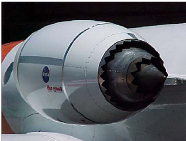
Fig. 5: Chevron nozzle flight test with Honeywell’s Falcon 20 test [13] .
