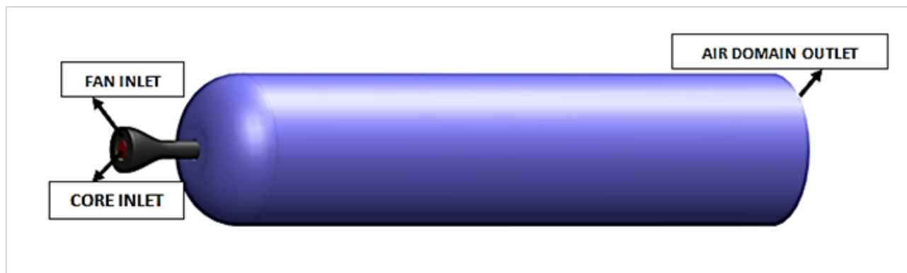
Fig. 10: Fluid flow domain with inlet and outlet boundaries
