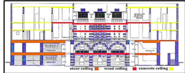
Fig. 26: An explanation of the different types of ceilings after the restoration process [13] .
