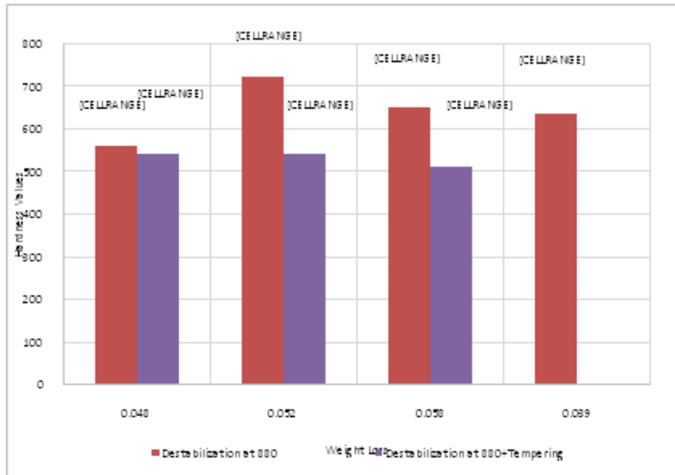
Fig. 10: The effect of the destabilization temperature at 880 °C Vs the effect of tempering on the mechanical properties for high chromium white cast iron
