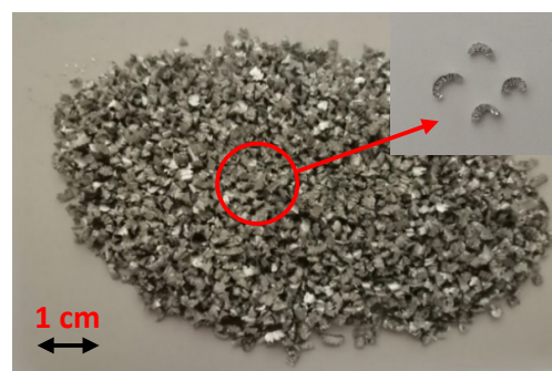
Fig. 1: Aluminum alloy 2011 chips
