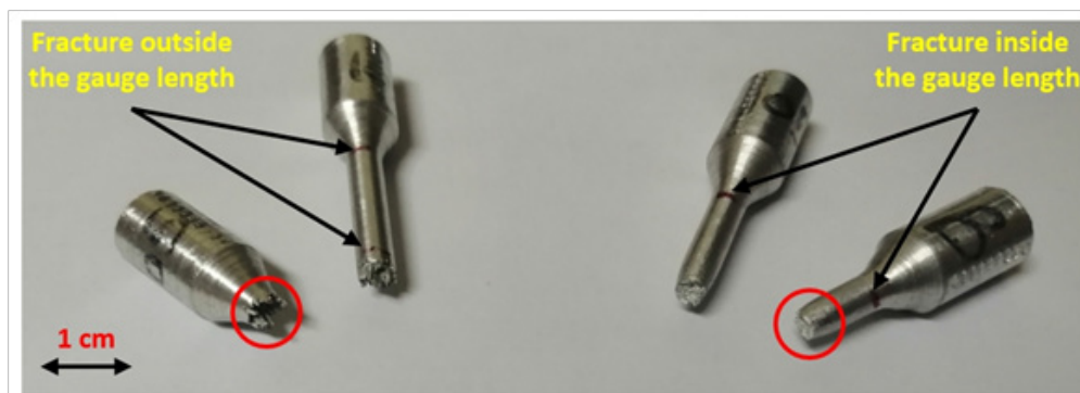
Fig. 6: Sample 9: specimen with brittle fracture (left) and specimen with ductile fracture (right)
