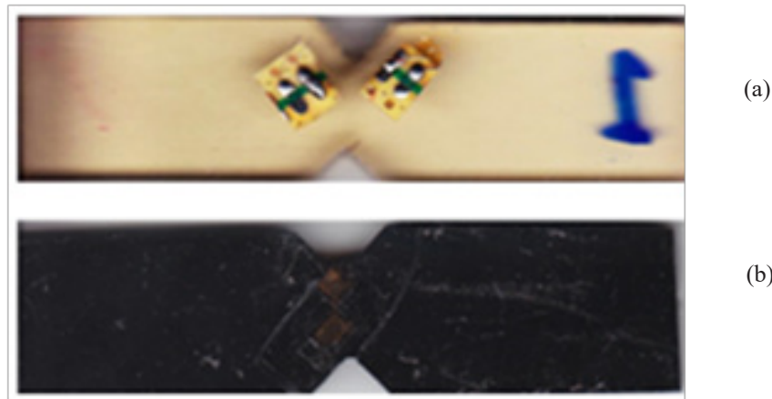
Fig. 14: Fractured specimens in shear test for : (a) NE, and (b) MWCNT-
