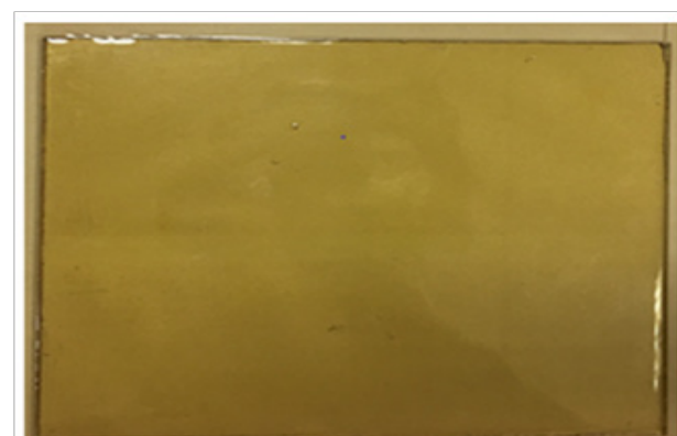
Fig. 1: Fabrication of neat epoxy panel: (a) Glass mold treated by liquid wax, and (b) The fabricated panel
