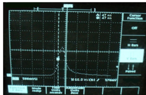
Fig. 6: Resolution of the main pulse in the Q-switched pulse packet at expanded time scale (60 ns/div).
