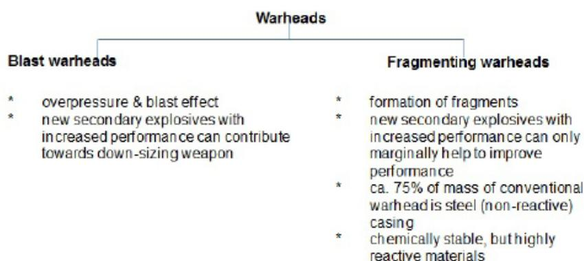
Fig. 1: Comparison of aspects of blast and fragmenting warheads (in addition to shaped charge warheads)
