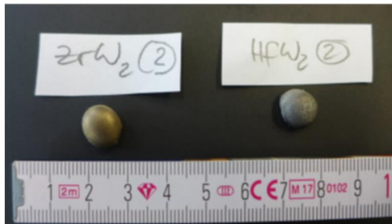
**Fig. 6:** Two samples of approximately 5 g of ZrW<sub>2</sub> and HfW<sub>2</sub>. ZrW<sub>2</sub> has a more “golden” color, whereas HfW<sub>2</sub> is silvery-metallic.
