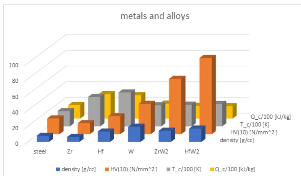
Fig. 6: Selected properties of metals and alloys
