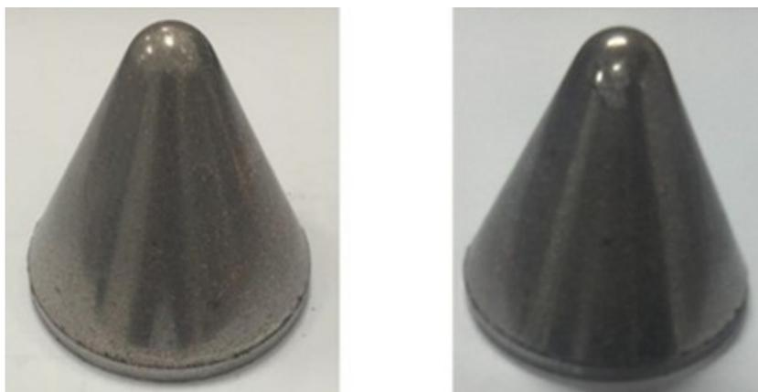
Fig. 4: A pressed (left) and sintered (right) PTFE/W/Cu/Pb SC liner.
