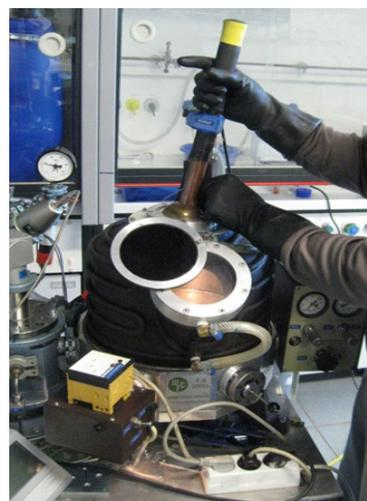
**Fig. 5:** Arc-furnace AF92-1000. The long copper electrode can be moved up and down and turned around by a circle-movement. Between the electrode and the outer casing of the arc-furnace there is a tension of about 15 V, therefore, the operator uses isolating gloves.
