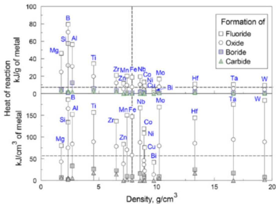
Fig. 3: Comparison of the heats of reaction for the formation of metal fluorides, oxides, borides and carbides<sup>[2]</sup>.
