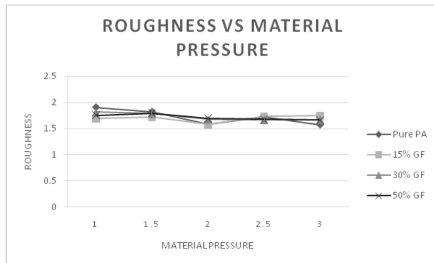
Fig. 2: Change in surface roughness (µm) with changing in material pressure (MPa)
