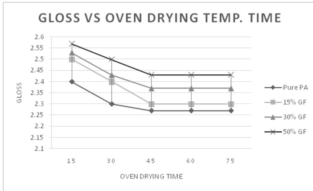
Fig. 7: Change in surface gloss with changing in oven drying temperature time
