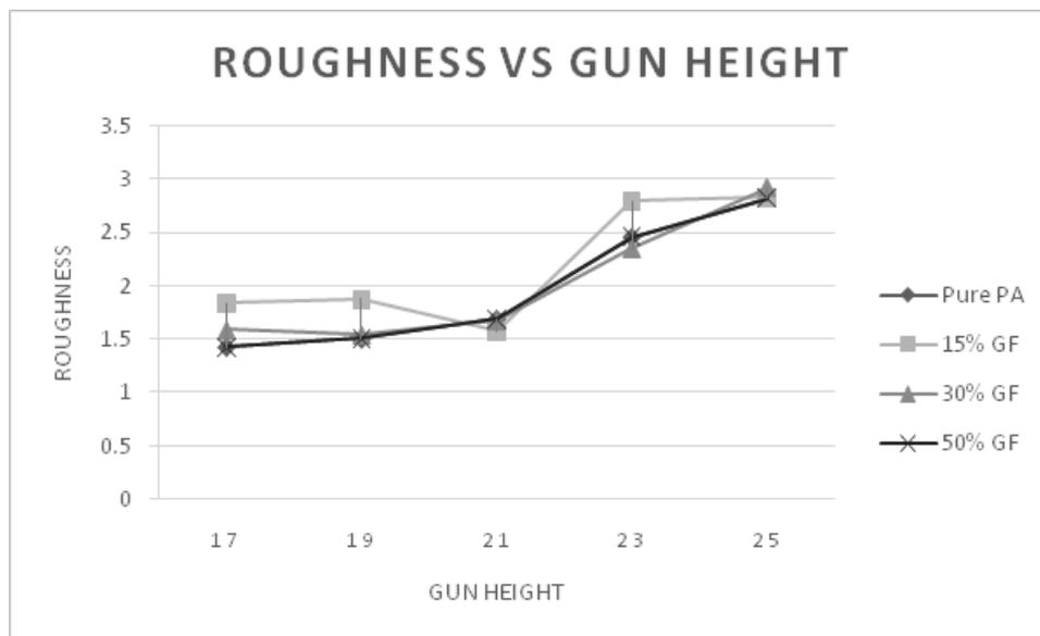
Fig. 4: Change in Surface Roughness ( $\mu\text{m}$ ) with Changing in Gun Height (cm)
