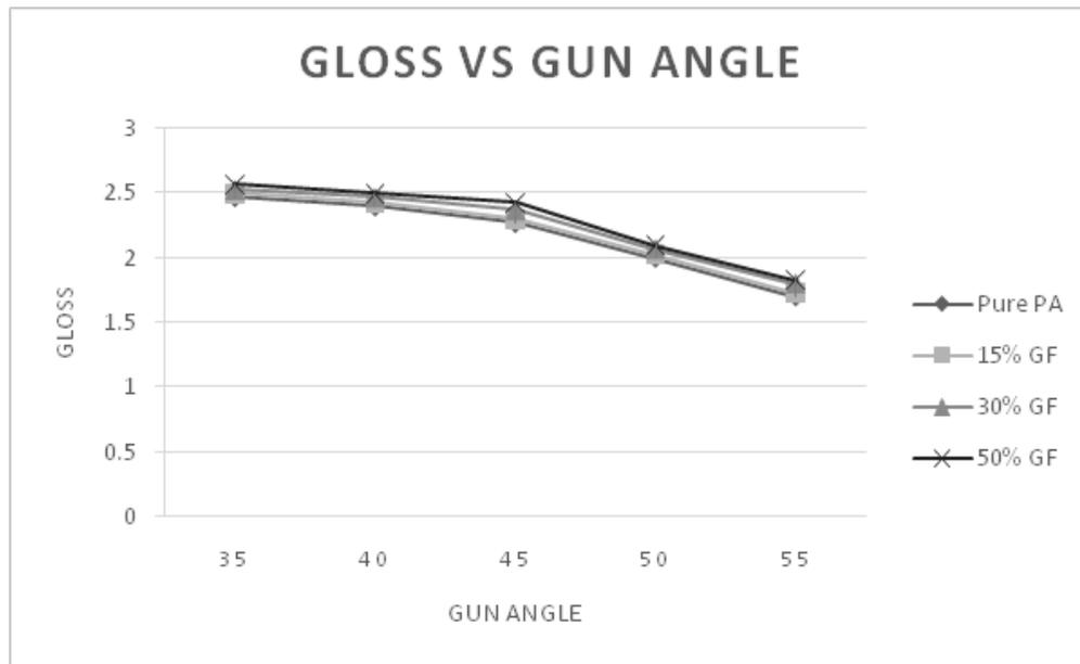
Fig. 9: Change in surface gloss with changing in gun angle
