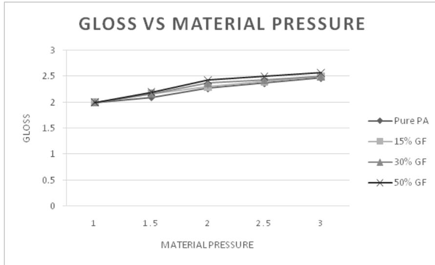
Fig. 3: Change in surface gloss (Gu) with changing in material pressure (MPa)
