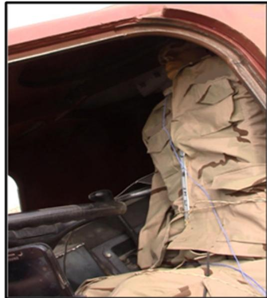
Fig. 11: Custom ATD seated on driver's seat inside the vehicle
