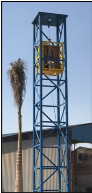
Fig. 5: Drop tower test facility for testing the custom ATD
