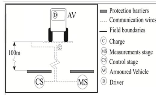
Fig. 8: A schematic drawing of test arrangement
