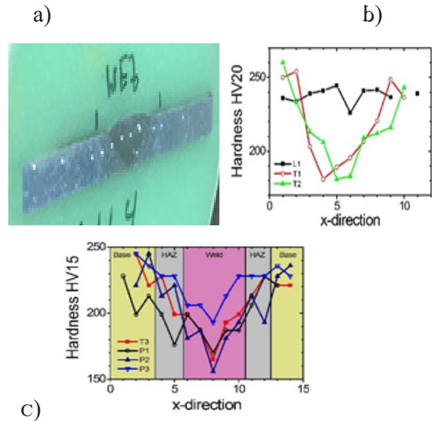
**Fig. 5:** Hardness evaluation at embedded welded sample with hardness indentations (a) and hardness profiles of the samples L1, T1, T2 (b) and T3, P1, P2, P3 (c). Regions of base material (base), heat effected zone (HAZ) and weld are indicated in (c).
