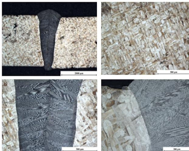
**Fig. 4:** Microstructure of laser welding of sample L1. (a) Overview with 2000µm scale bar, (b) base material with 500µm scale bar, (c) weld region with 500µm scale bar and (d) weld and HAZ with 200µm scale bar.
